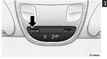
Use this button to change the display from U.S. to metric measurement units.
