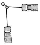
All winching operations should have a straight line from the winch to the object being pulled. This minimizes the wire rope collecting on one side of the drum affecting pulling efficiency and damaging wire rope. A snatch block, secured to a point directly in front of the vehicle will enable you to change your pulling direction while still allowing the wire rope to be at 90° to wind properly onto the spooling drum.
