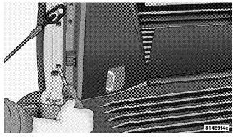
Removing the Two (2) Screws
