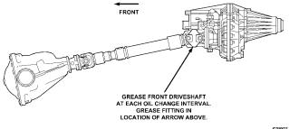
Front Driveshaft Grease Fitting
