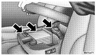
The center portion of the seat folds down to provide an armrest with unique storage compartments under the lid. Push the button on the front of the armrest to raise the cover. Inside there is a power outlet (if equipped), removable coin holder (if equipped), and two dividers to
