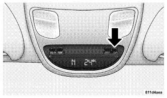
Use this button to select a readout of the outside temperature and one of eight compass headings that indicate the direction in which the vehicle is facing. UNDERSTANDING THE FEATURES OF YOUR VEHICLE 147
