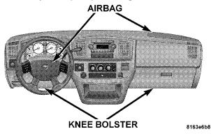
This vehicle has airbags for both the driver and right front passenger as a supplement to the seat belt restraint systems. The driver's front airbag is mounted in the steering wheel. The passenger front airbag is mounted in
