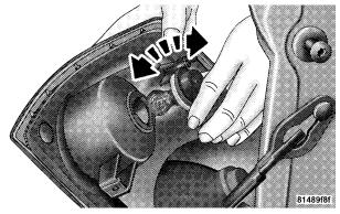
**Rotating Bulb Socket From Housing**
