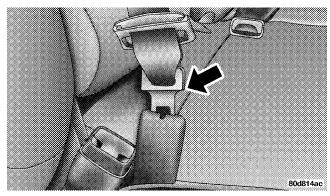
**Inserting Latch Plate**
