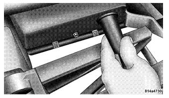
10. Put wire rope under tension. Using the remote control switch, slowly wind the wire rope until no slack remains. Once the wire rope is under tension, stand well clear and never step over it.
