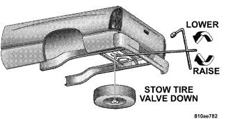
It is recommended that you stow the flat or spare to avoid tangling the loose cable. **NOTE:** The winch mechanism is designed for use with the jack extension tube only. Use of an air wrench or other power tools is not recommended and can damage the winch.
