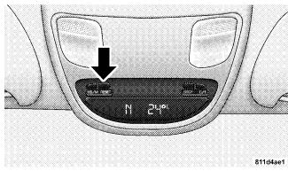
Use this button to reset the following displays: Average Fuel Economy (AVG ECO) Trip Odometer (ODO) Elapsed time (ET)
