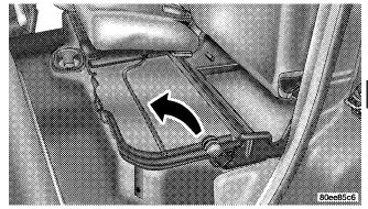
**Unfolding The Load Floor**
